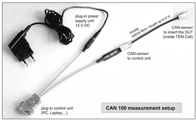
Figure 4 CAN 100 connected by 12 V adapter A01
