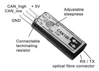
Figure 1 CAN 100 pin assignment
