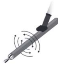
Figure 5: Near Field/H-Probe used to capture the radiated electromagnetic fields around an Ethernet cable.
