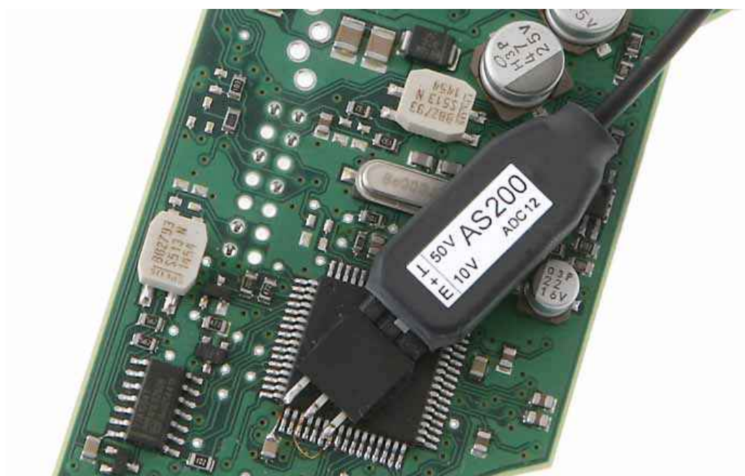
Application with AS 200 optical sensor
