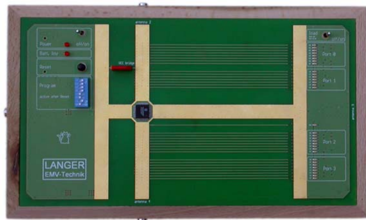
The VM 251 test board shows the effect of EMC measures on electronic devices.
