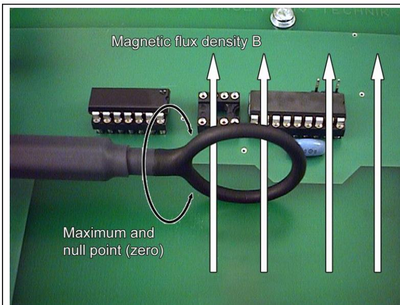
**Figure 5** Handling of MS 101 magnetic field probe
