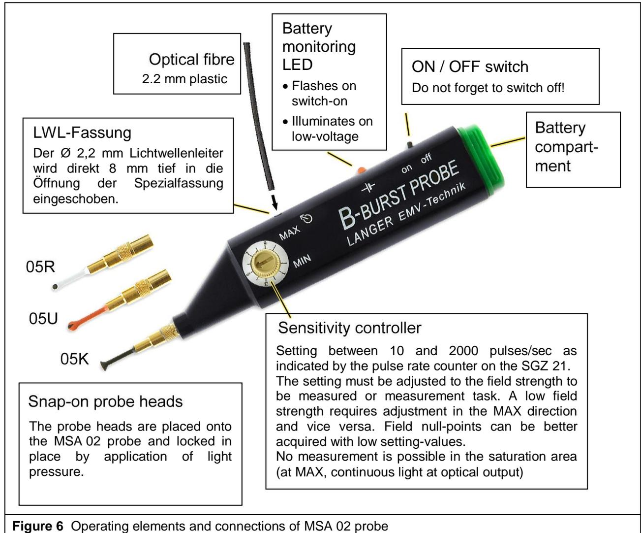
Figure 6 Operating elements and connections of MSA 02 probe
