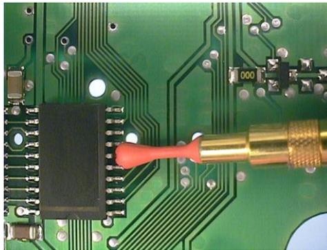
Placing the measuring groove onto surface / conductor.
