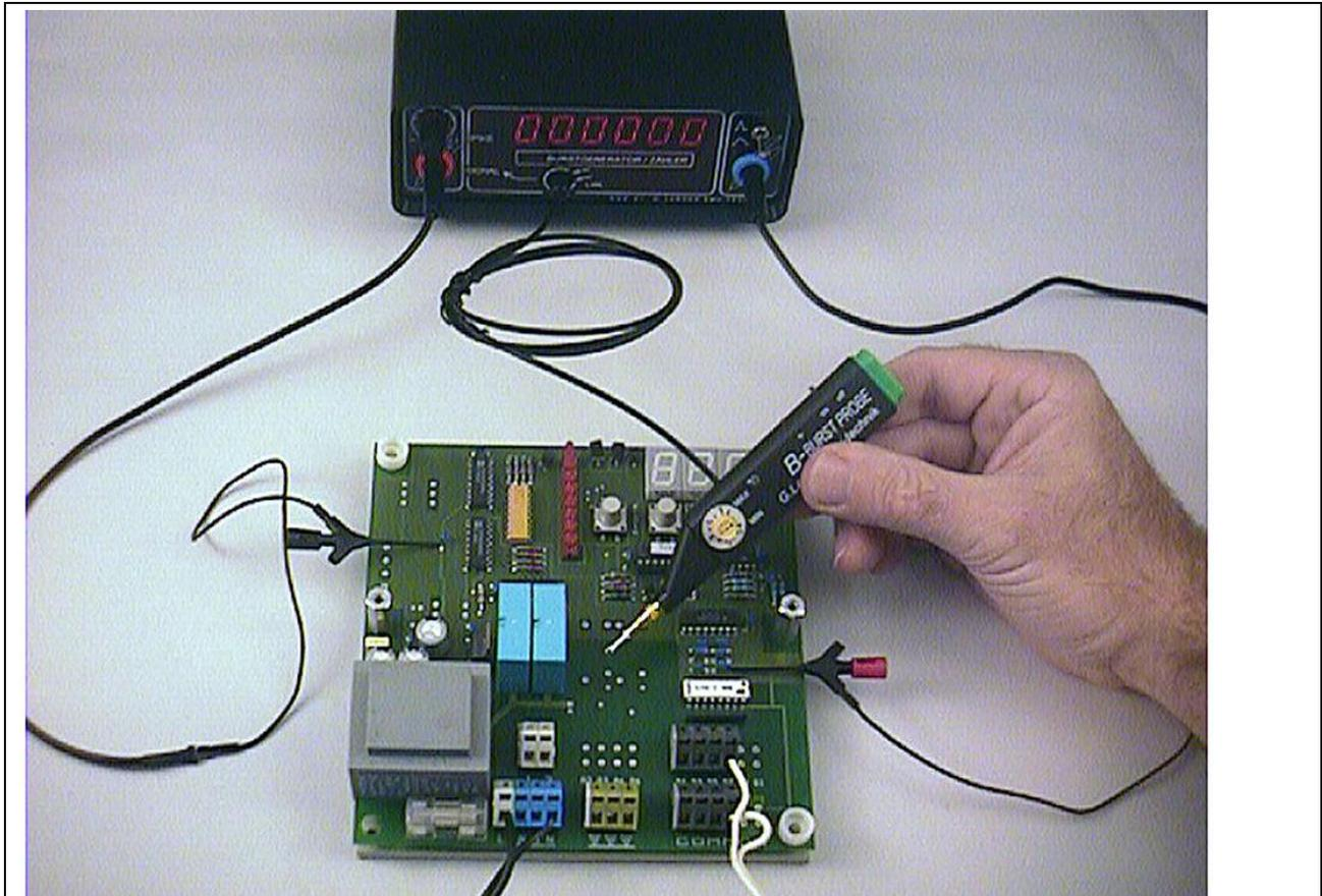
**Figure 10** Measuring station for pulse rate procedure
