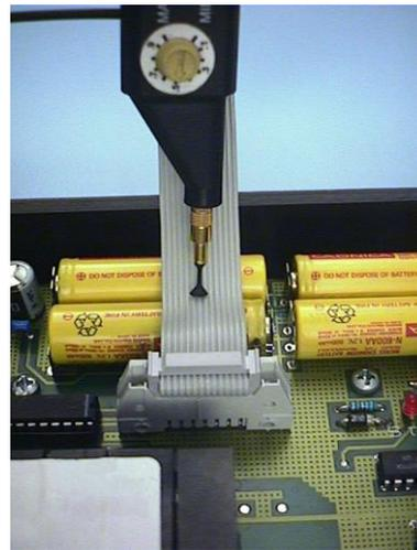
The circular magnetic field around conductors carrying pulse current can be selectively acquired with the 05K probe head. Homogeneous overlaid surface fields are not acquired by the probe.
