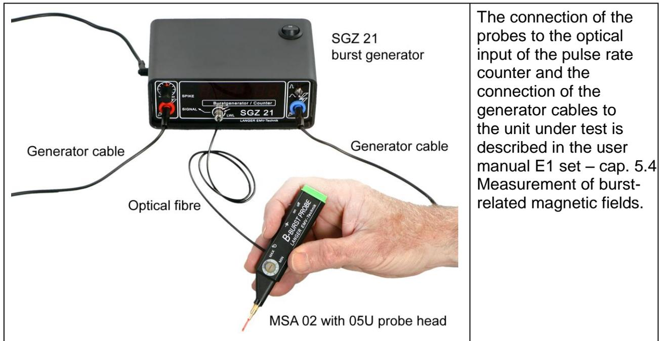
The connection of the probes to the optical input of the pulse rate counter and the connection of the generator cables to the unit under test is described in the user manual E1 set – cap. 5.4 Measurement of burst-related magnetic fields.
