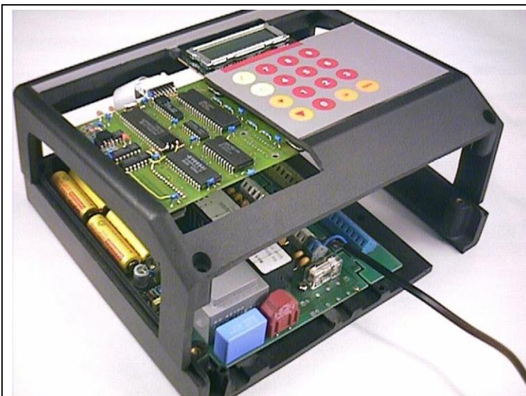
**Figure 11** If necessary, special openings must be made in the equipment case so that the measurement areas can be accessed with the probe.
