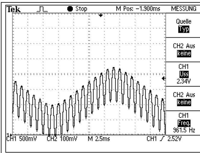
Figure 5 Useful signal with 1 kHz disturbance signal
