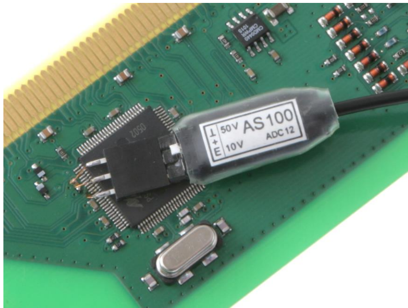
Figure 9 AS 100 connected to the DUT; position the AS 100 on the IC package if there isn't enough free space above GND
