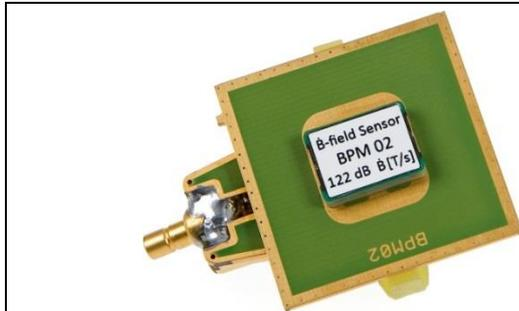
Figure 11 BPM 02 dB/dt field meter
