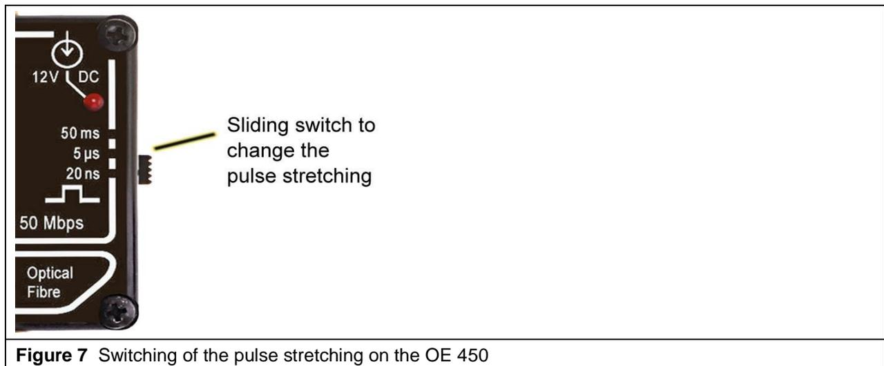
Figure 7 Switching of the pulse stretching on the OE 450
