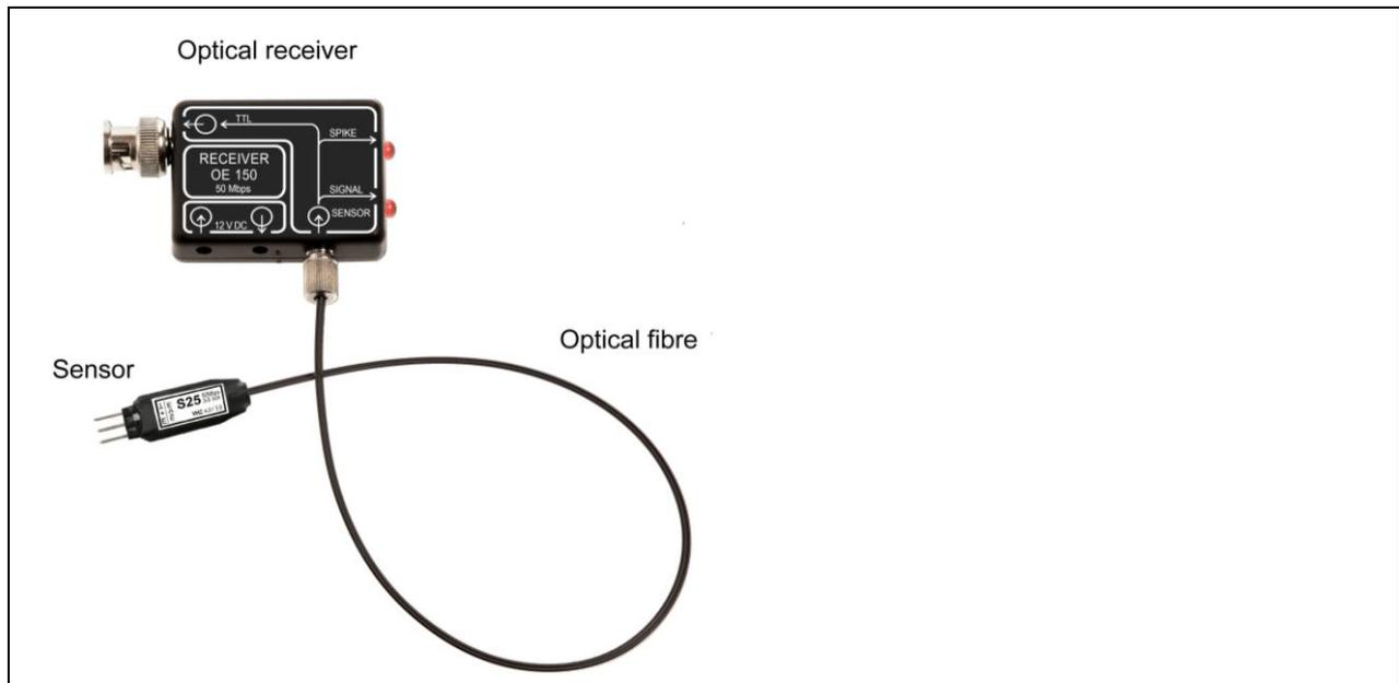
**Figure 1** Sensor, optical fibre and optical receiver are combined into a probe head
