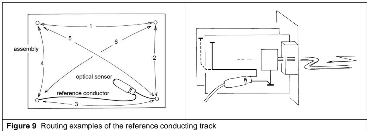
**Figure 9** Routing examples of the reference conducting track
