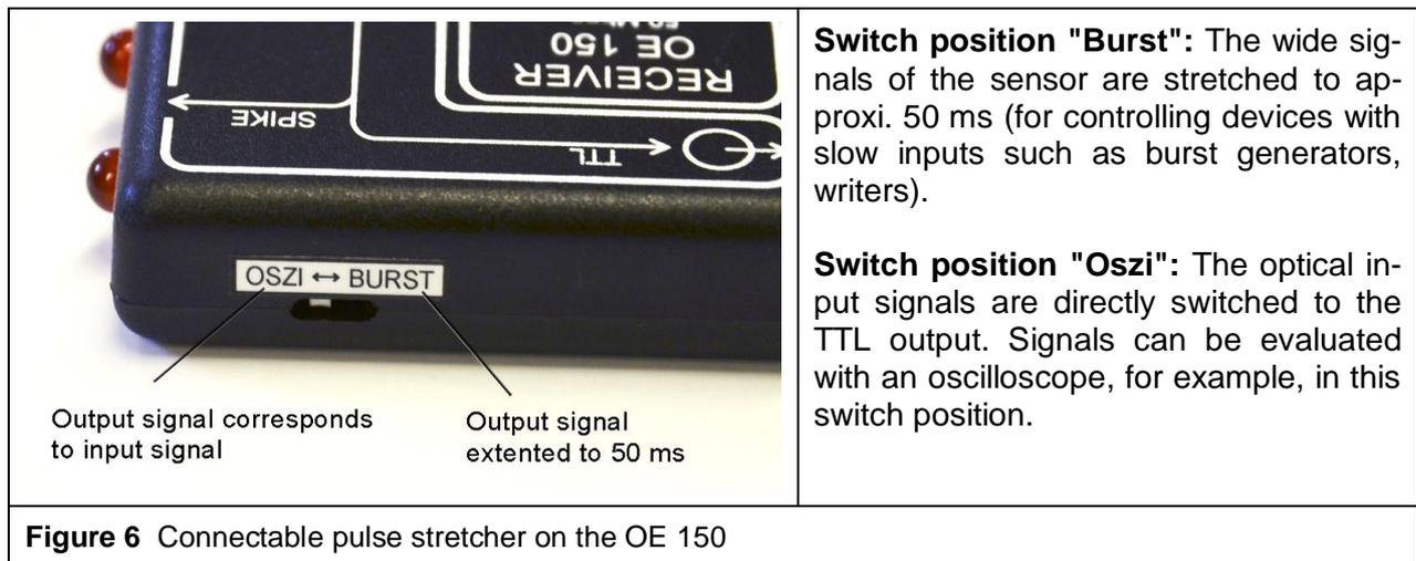
Figure 6 Connectable pulse stretcher on the OE 150
