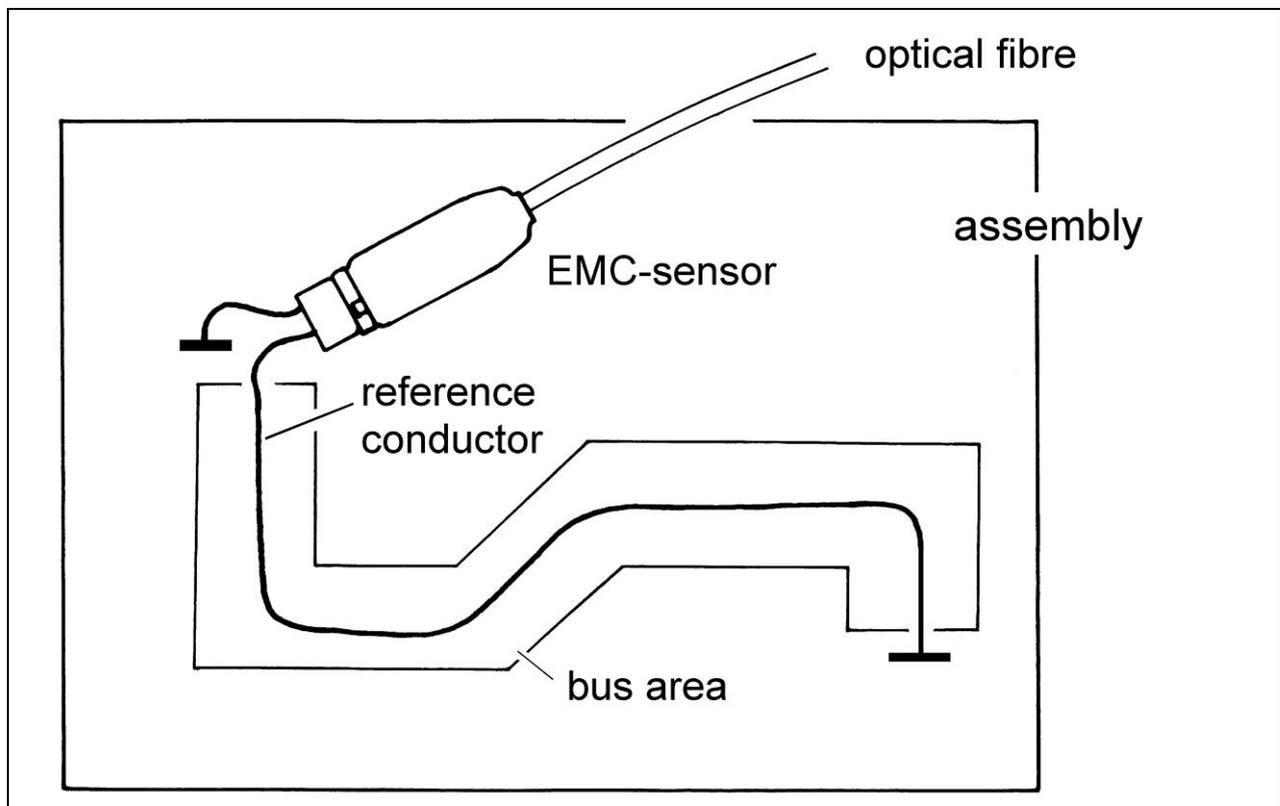
**Figure 10** Routing the reference conducting track with bus systems
