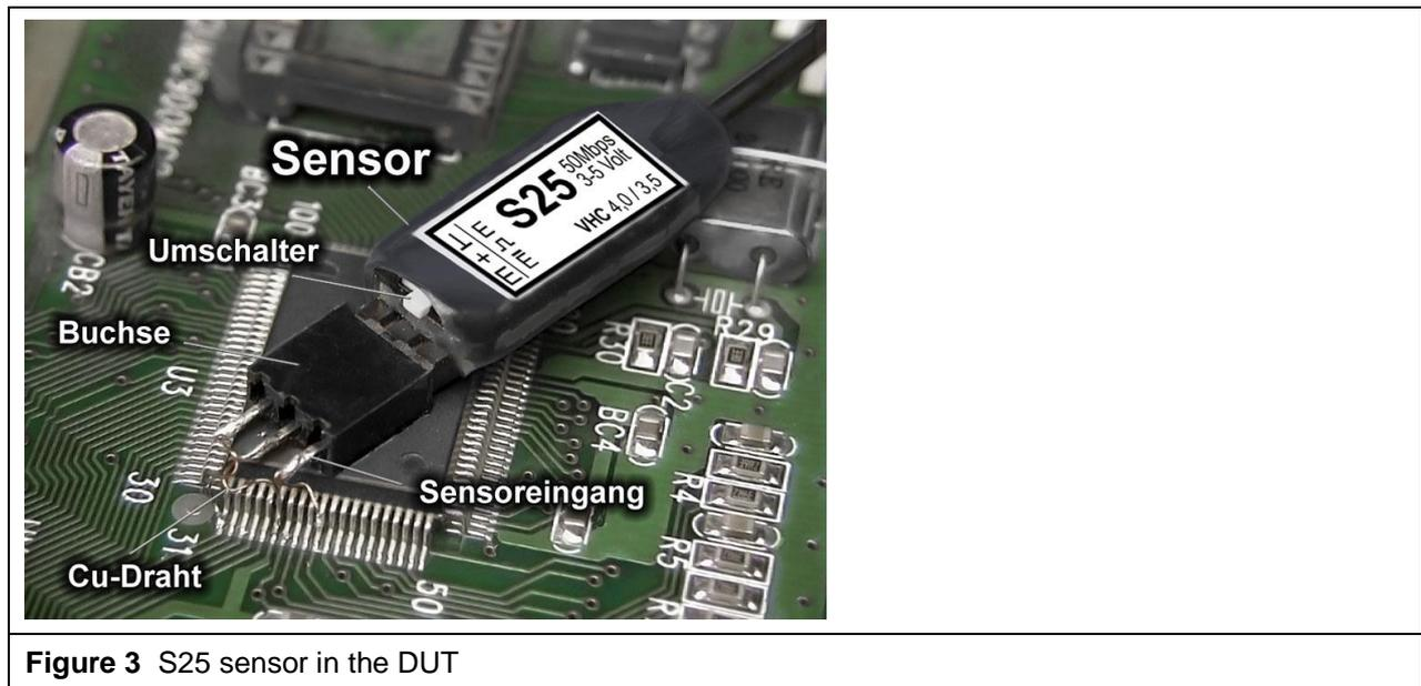
**Figure 3** S25 sensor in the DUT
