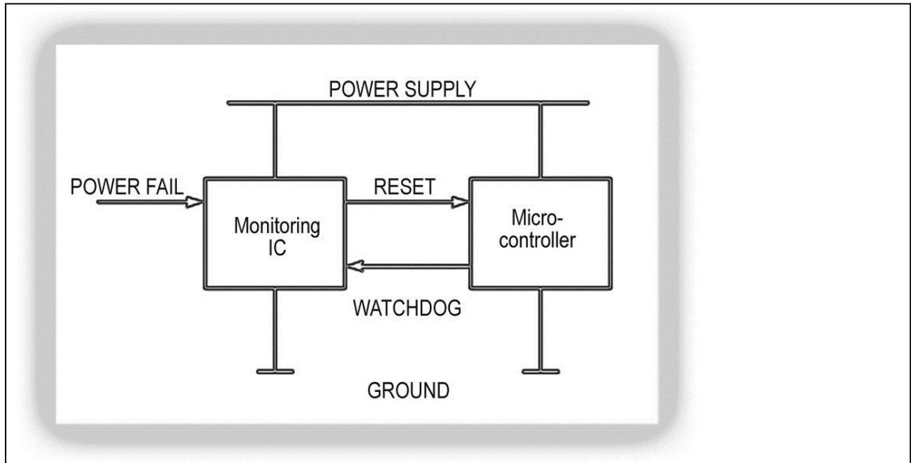
**Figure 11** Monitoring IC and microcontroller can cause a RESET
