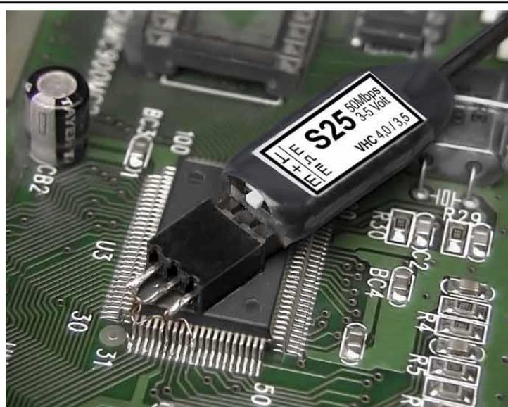
**Figure 2** S25 sensor integrated in the DUT
