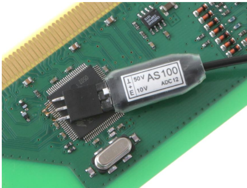
Figure 9 AS 100 connected to the DUT; position the AS 100 on the IC package if there isn't enough free space above GND
