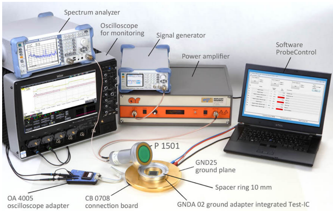
Measurement set-up with P1501 RF E-Field source
