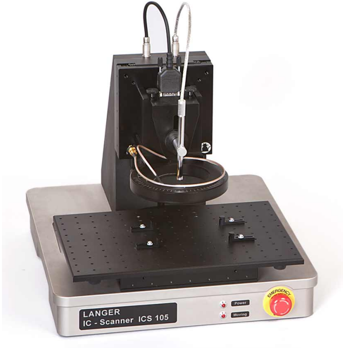
ICS 105 set with UH DUT universal holder and device under test
