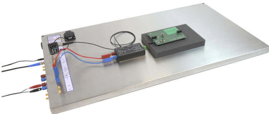
SA 21 demo board with RF-R 400 near-field probe on cable
