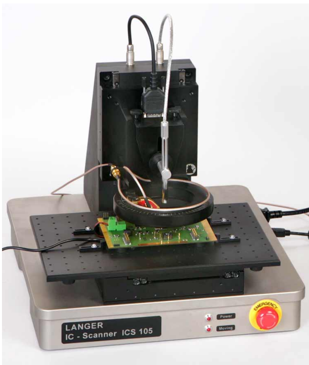
ICS 105 set with UH DUT universal holder and device under test
