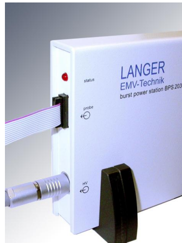
Figure 28: Connecting the BPS 203 to the probe
