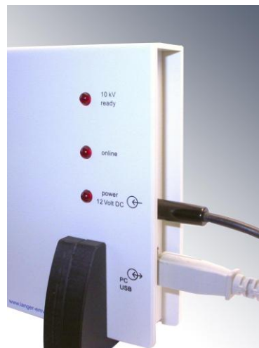
Figure 27: 12 V power supply unit and USB ports
