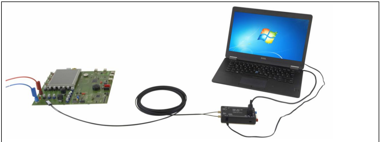
Figure 7: One sensor with one Opto-Box for data transmission without LIN/CAN bus cable
