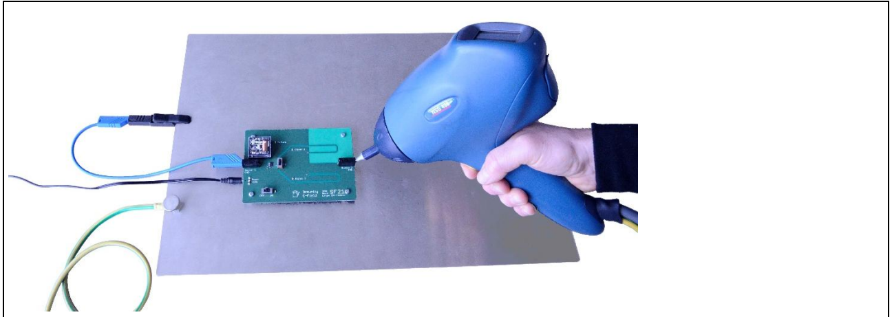
Figure 21: Experiments with ESD generator over a metal surface
