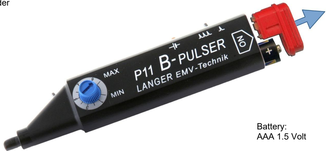
Figure 2: Changing the battery of the Mini Burst Field Generator
