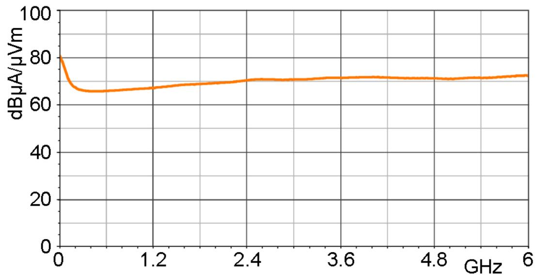
Korrekturkurve Strom [ $\text{dB}\mu\text{A}$ ] / [ $\text{dB}\mu\text{V}$ ]
