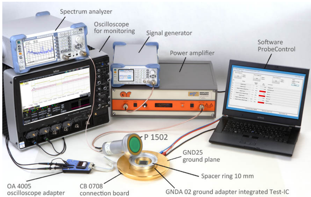
Measurement set-up with P1502 RF E-Field source
