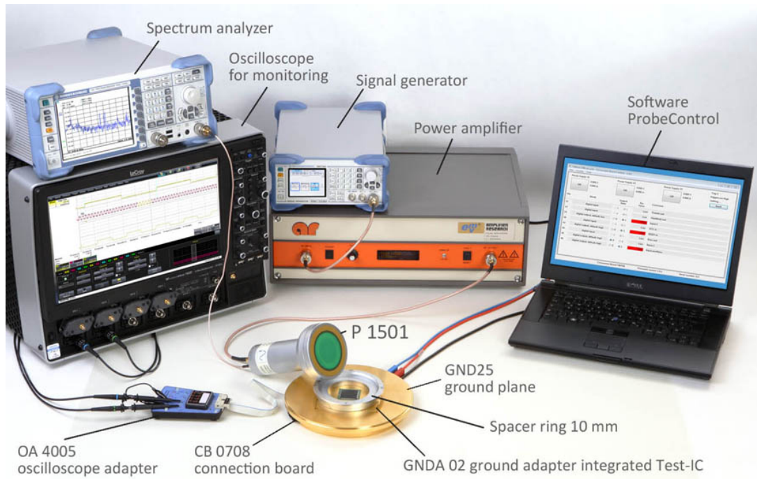
Measurement set-up with P1501 RF E-Field source
