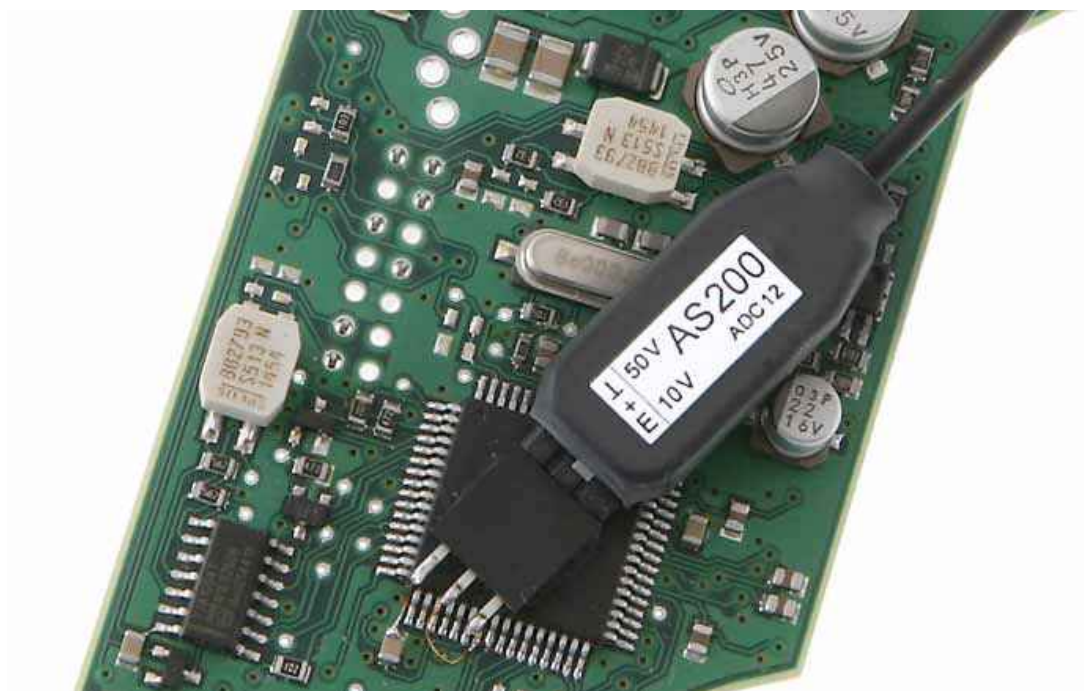
Application with AS 200 optical sensor
