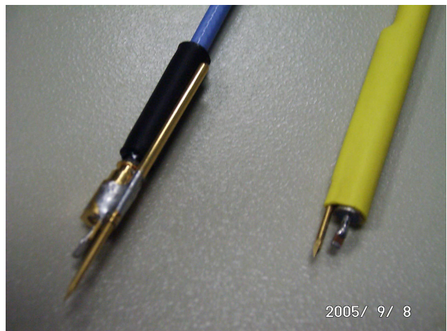
Fig. 5 Test fixture with optimal flexibility to inject EMS RF signal on a dedicated pin of the DUT.
