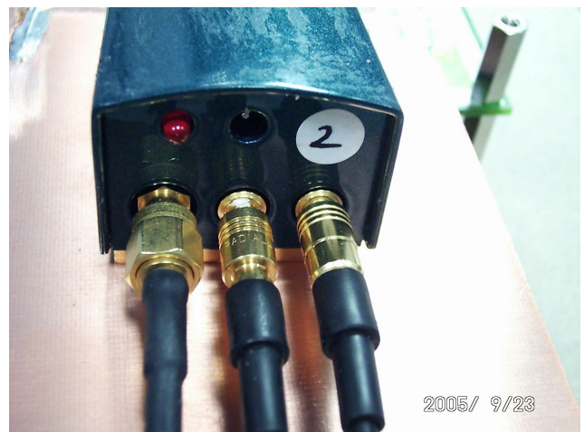
Fig. 15 Rear panel of RF injection probe with connectors for RF power, RF current and RF voltage measurement.
