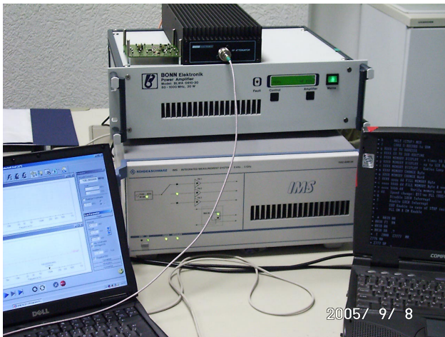
Fig. 7 IMS station ( R&S, Germany) equipped with additional external 30Watt power amplifier (Bonn Elektronik, Germany) represent the EMS measurement components. Screen on the lower left side shows control panel of IMS station. Screen on the lower right corner monitors results from the DUT under RF signal violation.
