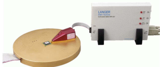
Figure 3: Burst measurement setup with IC under test, test board, probe 201 and burst power station.
