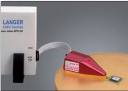
Figure 2. System for testing IC immunity to pulse disturbances
