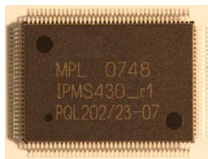
(a) QFP with pins on all sides
